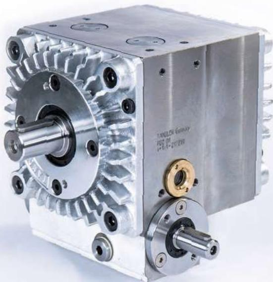
*The PD2 is a double planetary gear with internal gear ratios of  $i_1=1:3$  and  $i_2=3:1$ , whereby the rotational speed is modulated on one of the two ring gears. The second ring gear is fixed. The backlash between the worm and the worm gear can be minimized and adjusted by the adjustable cam position of the worm.*
