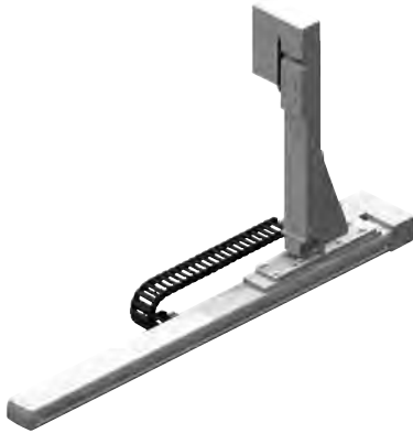
Wiring 1 with cable track
